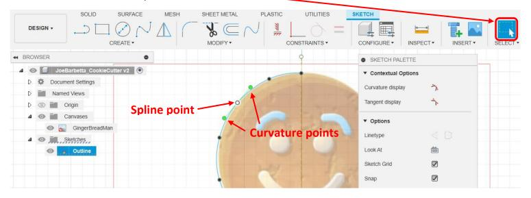
There are some irregular curved sections where a Spline is the most useful. However, an alternative for a section that is circular, an arc can be used.
